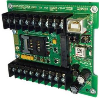
Figure 1: Flexi1 in its basic form, includes optional communications flexi card.
