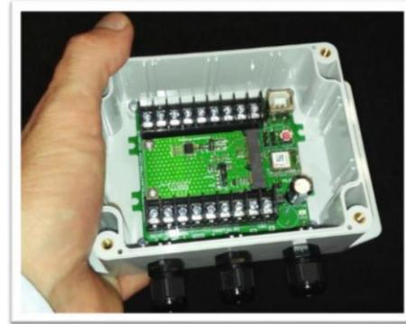
Figure 2: Flexi1 provided with optional IP67 rated enclosure and battery pack.
